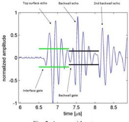
Fig. 2. A-scan with gates
