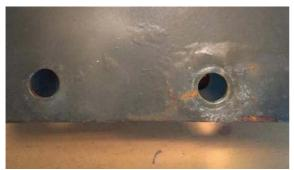
Fig. 5. Corroded element
