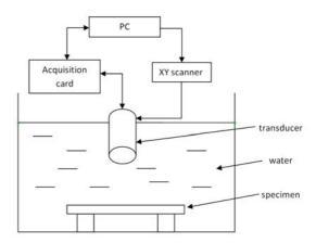
Fig. 3. Equipment setup
